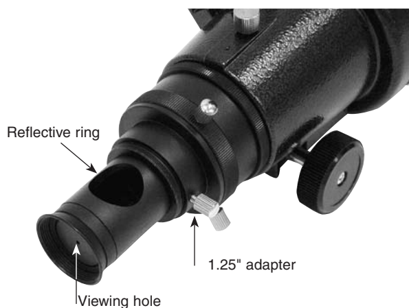
Figure 6-1. The collimating tool in the StarSeeker 100 focuser.
